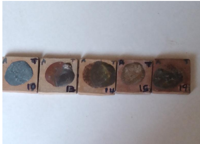
Fig. 12: Glaze A: The rough glazed samples (10, 13, 14, 15, and 19)
