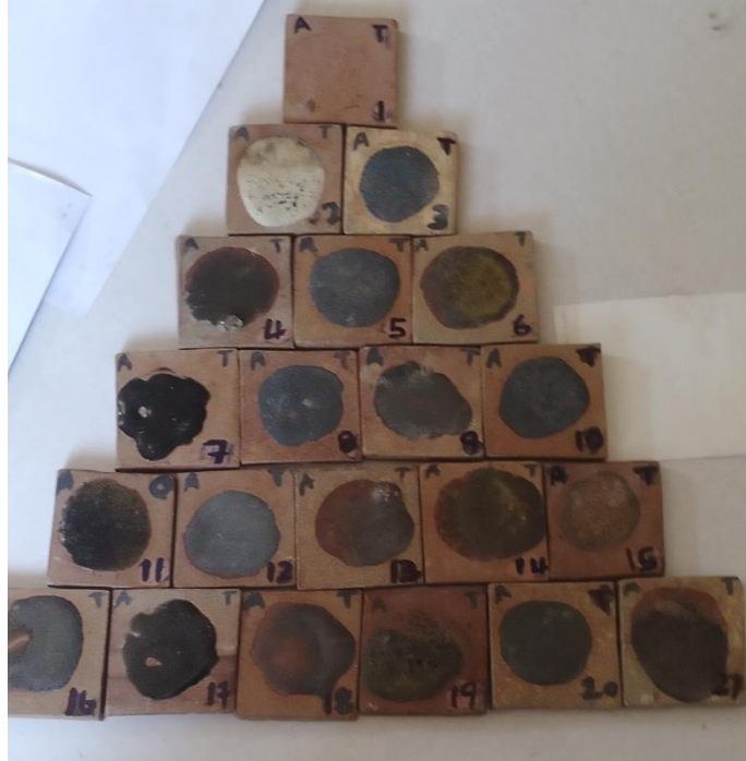
Fig. 6: Triaxial blend of Glaze A: Granite Dust (GD), Feldspar (F), and Iron Oxide (IO)
