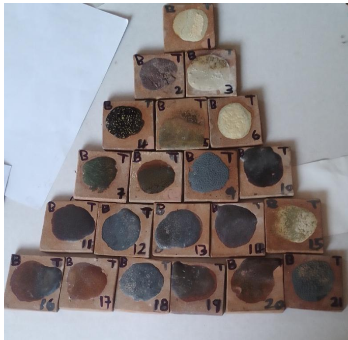
Fig. 7: Triaxial blend of Glaze B: Commercial Silica (CS), Feldspar (F), and Iron Oxide (IO)
