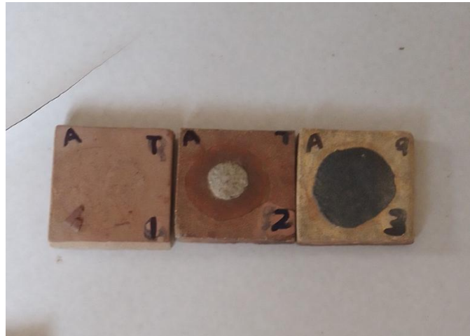
Fig. 10: Glaze A: The incomplete melting glazes (1, 2 and 3)
