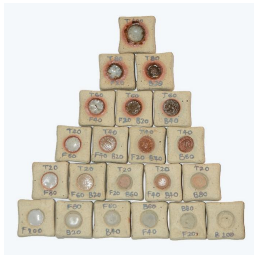
Plate 10: Triaxial Blend Comprising Tiger Nut Chaff Ash and Feldspar
