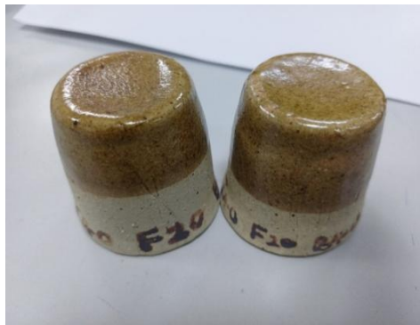
Plate 2: Stoneware fired at 1260°C with glaze formular TCNA 40% Potassium Feldspar 20% Ball clay 40% Source: Research Photograph, Aigbudume (2025)
