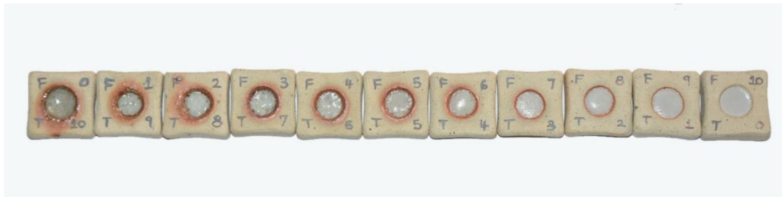
Plate 9: Line Blend Comprising Tiger Nut Chaff Ash and Feldspar
