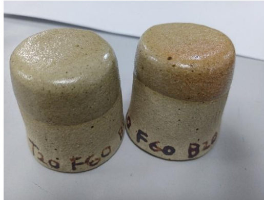
Plate 3: Stoneware fired at 1260°C with glaze formular TCNA 20% Potassium Feldspar 60% Ball clay 20% fired at 1260°C
