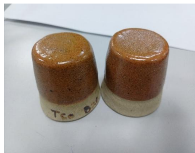
Plate 1: Stoneware fired at 1260°C with glaze formular TCNA 60% Potassium Feldspar 20% Ball clay 20%
